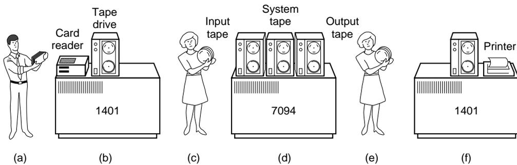
**Figure 1-1.** An early batch system. (a) Programmers bring cards to 1401. (b) 1401 reads batch of jobs onto tape. (c) Operator carries input tape to 7094. (d) 7094 does computing. (e) Operator carries output tape to 1401. (f) 1401 prints output.
