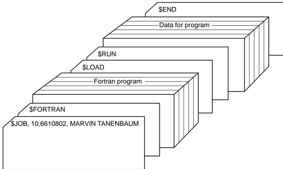
**Figure 1-2.** Structure of a typical FMS job.
