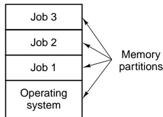
**Figure 1-3.** A multiprogramming system with three jobs in memory.
