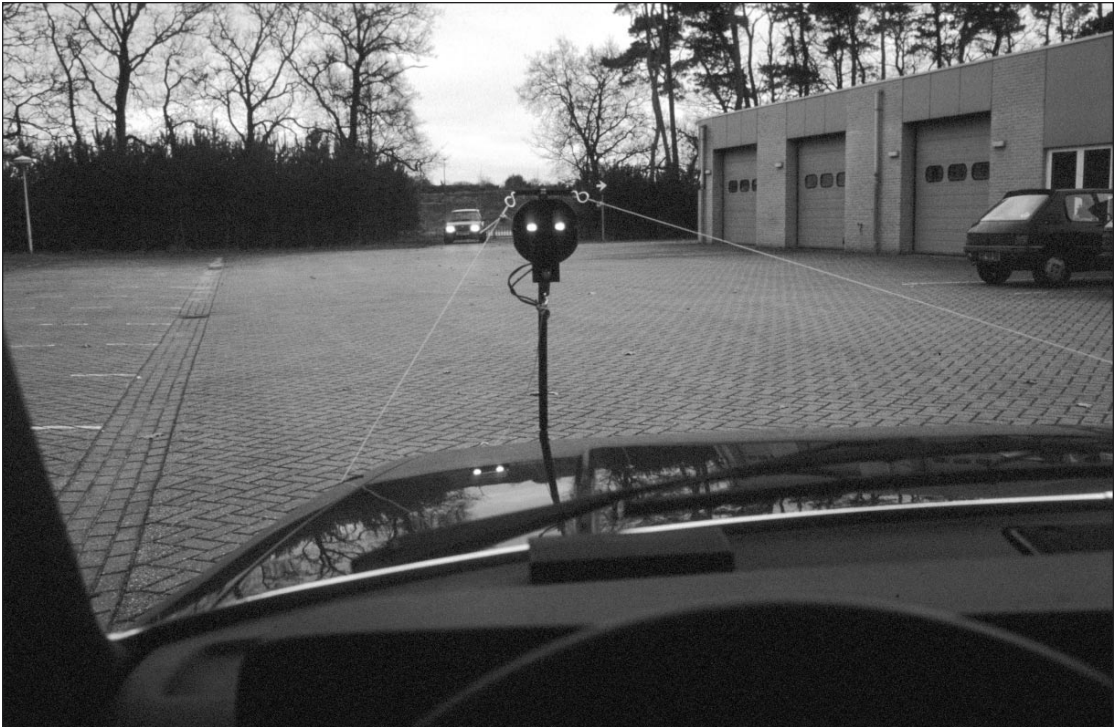
Figure 1. The view from the position of the driver. To the left is an actual car, to the right is the lighting rig.
