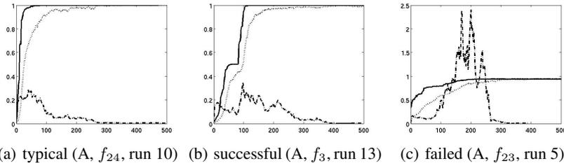
**Fig. 3.** Three examples of breeders’ evolution and response to premature convergence. Lines represent best fitness (solid), mean fitness (dotted) and mutation step size for candidate solutions (dashed) over time.
