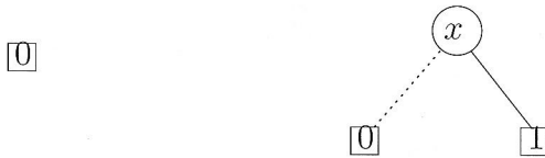
Figure 6.6. The BDDs (a) B_0 , representing the constant 0 boolean function; similarly, the BDD B_1 has only one node 1 and represents the constant 1 boolean function; and (b) B_x , representing the boolean variable x .
