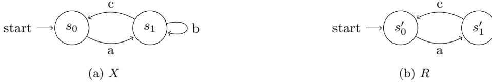
Figure 3.1: Automata of our running example  $X$  and its required external behaviour  $R$
