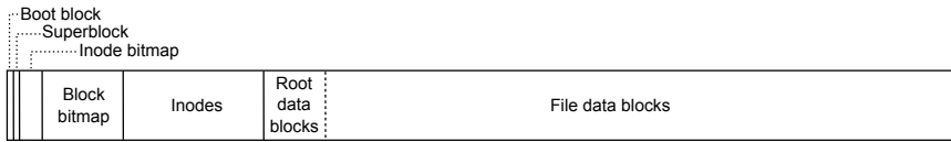
Figure 2.2: High-level overview of the on-disk layout used by the physical layer prototype.
