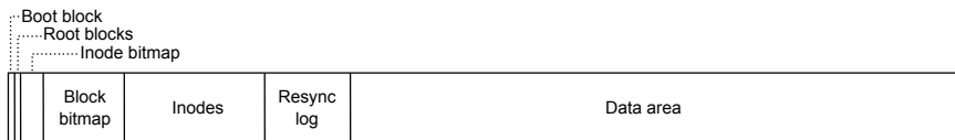
Figure 3.3: High-level overview of the TwinFS on-device layout. The root, inode, and bitmap blocks are metadata and thus protected. The data area contains both protected and unprotected data blocks, as well as indirect blocks, which are metadata and thus protected. The resynchronization log is described in Sec. 3.5.3.
