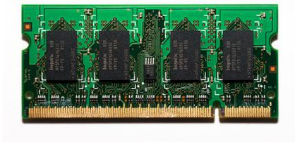
Figure 2: A SO-DIMM with its memory chips.
