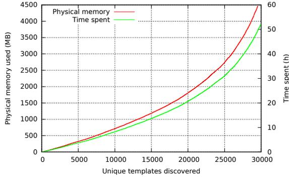
Figure 4: Required time and memory for templating.
