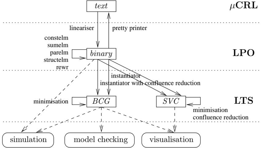
Fig. 1. The main components of the  $\mu\text{CRL}$  toolset
